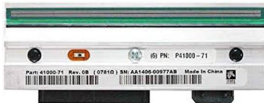
Thermal printhead is a linear array of resistors 150 to 600 per inch
