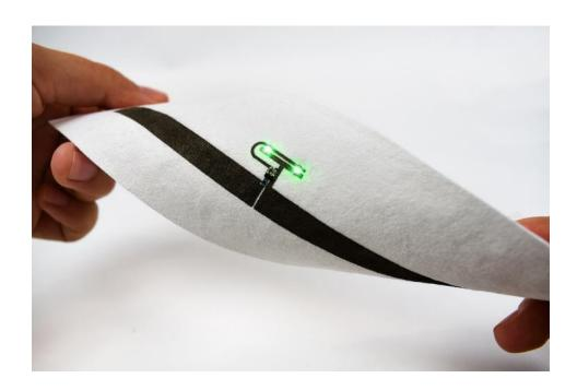
Textile printed circuitry that is fully waterproof, flexible, and wirelessly powered.
