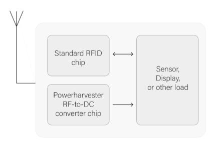
Existing RFID infrastructure can be used dually as a wireless power delivery system
