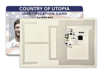
Integration of RF power harvesting technology removes or reduces the need for a battery, allowing the card to remain ultra thin while supporting additional advanced features.
